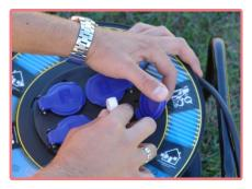
Plug with extention can be secured by inserting into the airgate.
